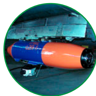
Cameras/sensors housing pod LZR-1 (recorders)
